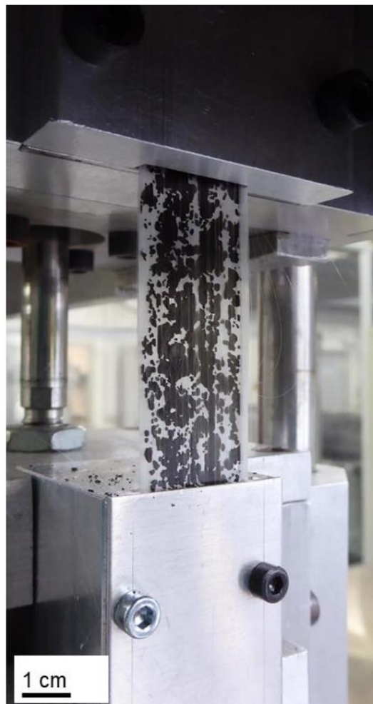
Figure 45: Tape guide with a width of 20 mm on the IVW's universal laying head
