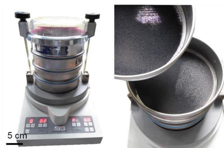
Figure 34: Sieving of polymer material into different size fractions
