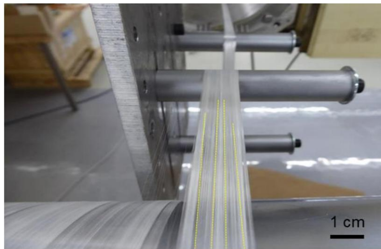
Figure 37: Unequal filament distribution with a large spreading width
