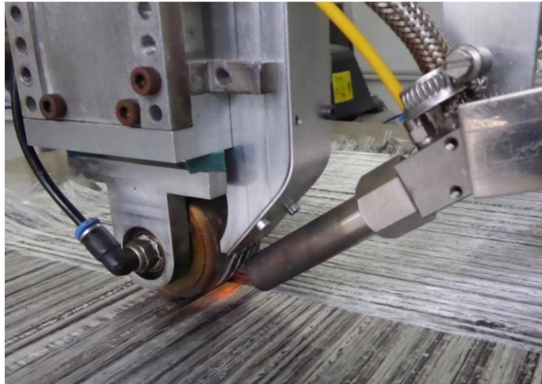
Figure 47: Depositing the PowderTapes into preforms with a hot gas nozzle
