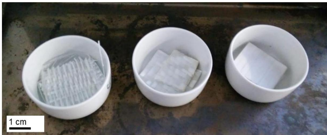
Figure 22: Glass fibers remaining after incineration (right: PowderTapes project)
