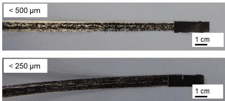
Figure 46: Tapes produced with different grain size distributions of the thermoplastic powder
