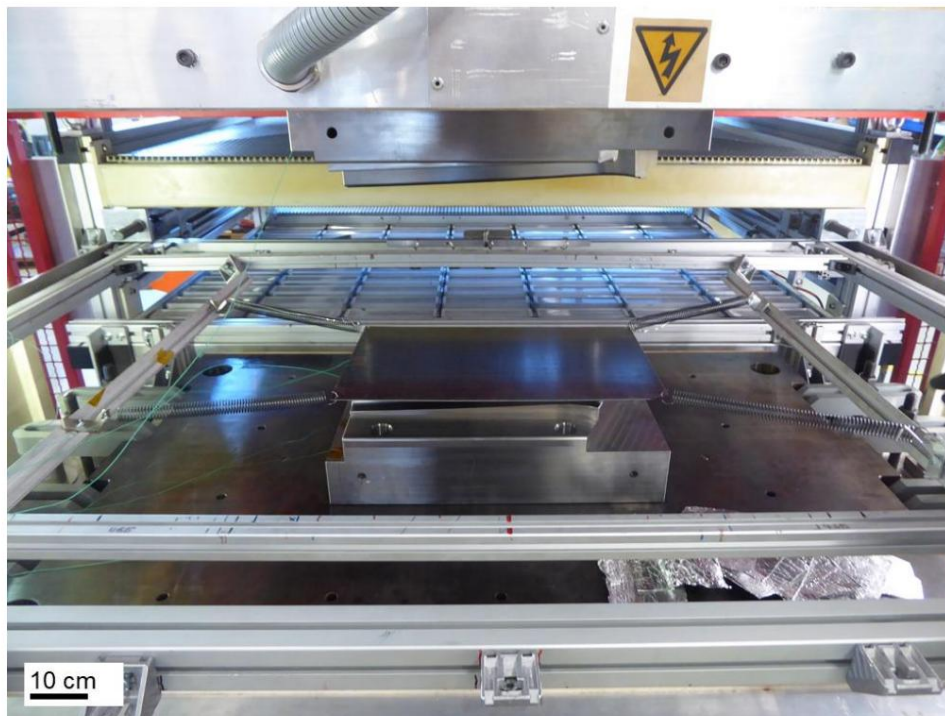
Figure 13: Organo sheet fixed in the transfer frame
