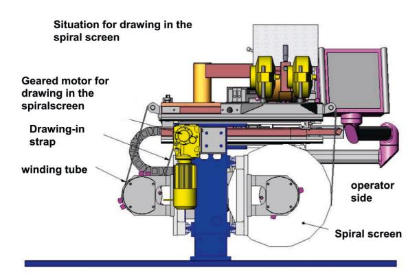
Before the semi-automatic filling process starts, the rear and front winding drive are positioned via the manual control in such a way that the right screen edge (seen from the operator side) is aligned with the table edge.
