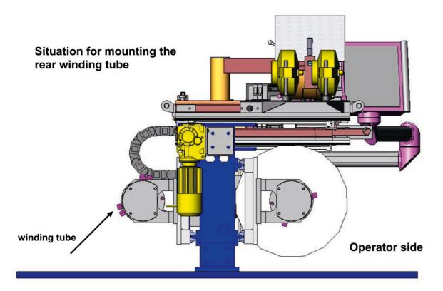
After retracting the table plate, the spiral screen to be filled which is wound up on a winding tube is inserted on the operator side.
